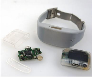
**Figure 3.** Wearable sensing platform for recording climbing activities that consists of a high-resolution tri-axial accelerometer, OLED screen (not used), on-board processing unit (PIC), battery, and flash memory.
