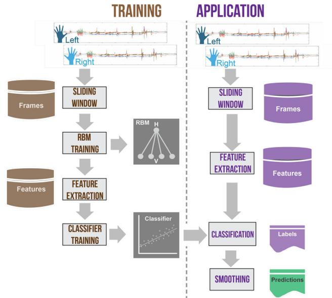
**Figure 4.** Overview of climb detection procedure: Sliding window frame extraction and feature learning (using Restricted Boltzmann Machine – RBM) for capturing characteristics of movement patterns, which are classified using statistical classification backend.
